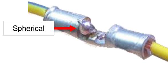
✗ Figure 13 (Spherical solder, soldering iron not hot enough)
