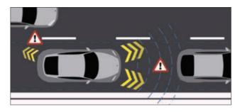
The altered refraction of the radar waves can severely limit performance and precision.
