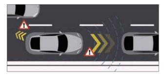
Radar waves can be deflected or dampened.
