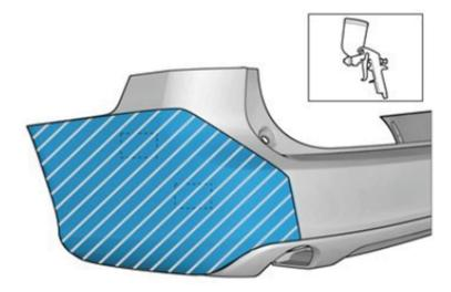
Note! Only one layer of metallic paint may be applied in the marked area.
