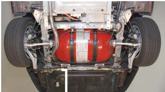
Hydrogen Pressure Relief Tube Location
