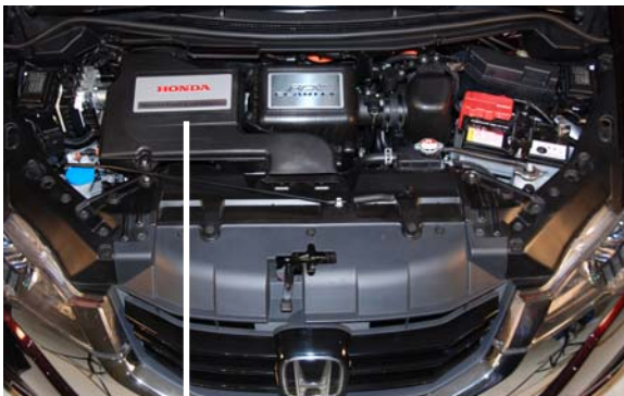
The Power Drive Unit (PDU) is located under other components and can be reached only by their removal.
