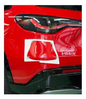
To assist technicians in determining where the radar wave emission area is, a printable template is provided in the body repair manual. This template can be taped onto the bumper and will help determine if the bumper can be repaired or will require replacement.
