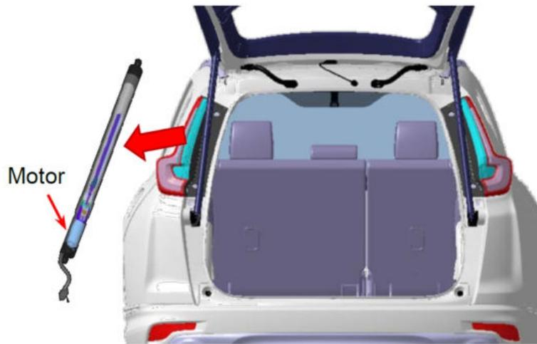
Spindle-Type Power Tailgate Actuator
