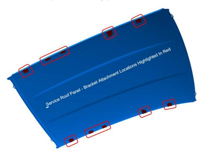
Service Replacement Roof Panel (Underside View)
