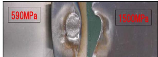
Tensile Test Results of Welded 1,500 MPa Steel
