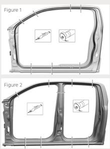
These illustrations are intended as a general guideline for door-opening panels (DOP) and are not all-inclusive. As a general rule, the grade of steel and location on the vehicle determines if structural components can be sectioned. Components constructed of dual-phase (DP 800) or higher strength/ grade steel should **not** be sectioned.
