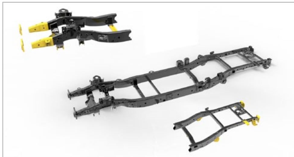
The fully-boxed frame of the new 2015 Ford F-150 helped play a big role in the truck earning an overall 5-Star crash safety rating. Engineers increased the amount of high-strength steel from 23 percent to 77 percent, which not only increased the material's stiffness but allowed it to be up to 60 pounds lighter. The frame, seen here with its separately serviceable parts highlighted in yellow, has front-third (PN# FL3Z5019H) and rear-third (PN# FL3Z17N775D) sections available to repairers.
