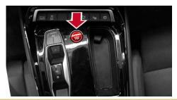
Press the START-STOP button without depressing the brake pedal
