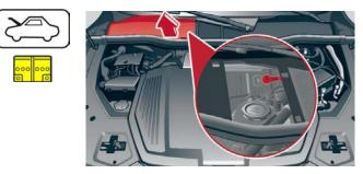
The 12-volt battery is located at the front of the vehicle under the plenum chamber cover.
