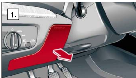
Fuse box – left-hand drive (steering wheel left)
