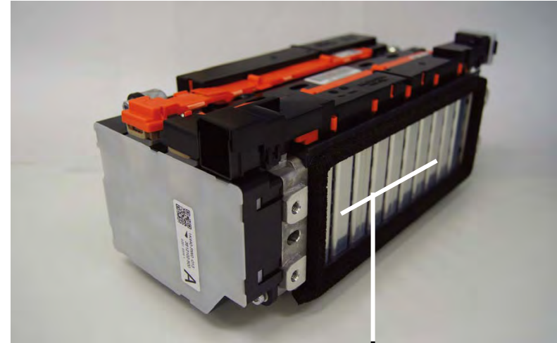
One of Four Battery "Stacks"
