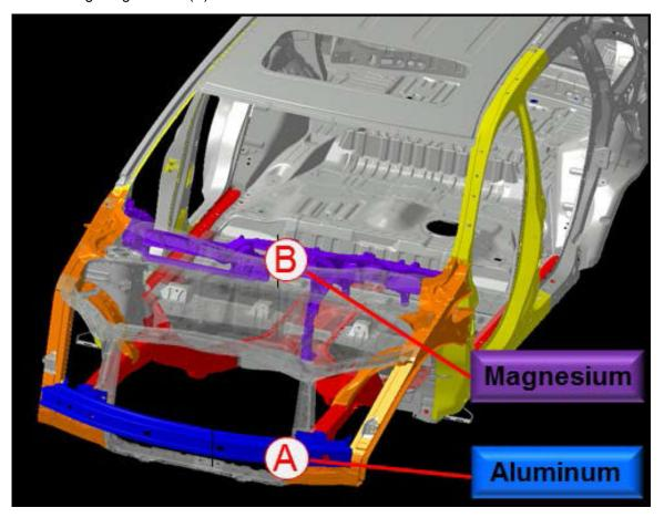
Do not attempt to repair magnesium parts and aluminum bumper reinforcement beams if damaged.
