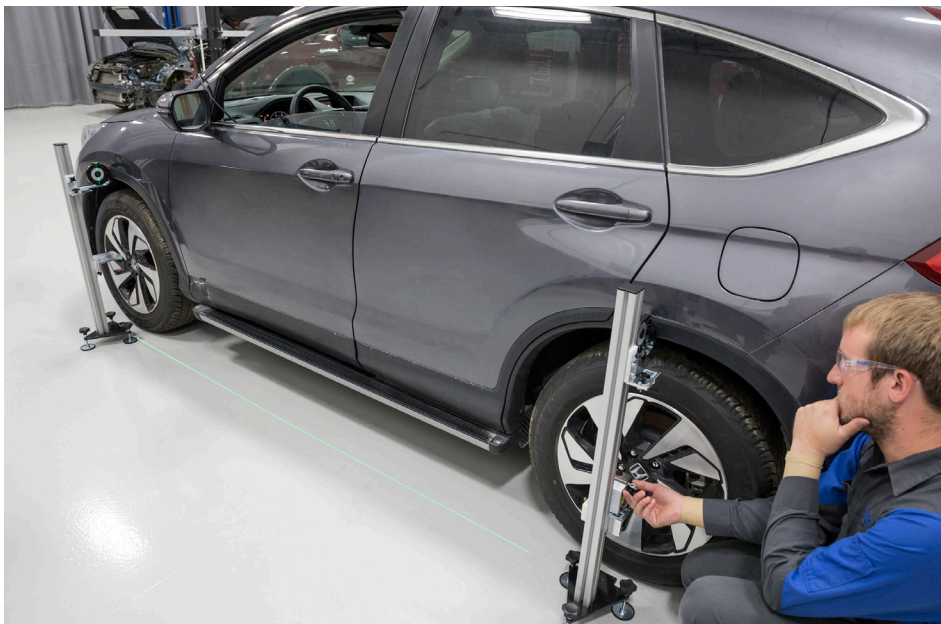
Forward-facing camera calibration set-up on a Honda CR-V.
