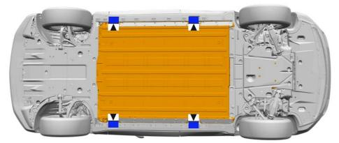
Make sure to remove the Rocker Panel Molding Jacking Opening Front Cover before positioning the lift onto the vehicle.
