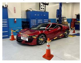
When removing the high-voltage battery, designate an area of the shop where it can be safely stored during repairs. A buffer zone should also be created, and cones placed for safety.
